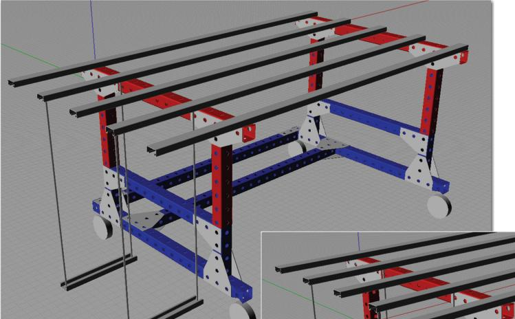
ADJUSTABLE STANDING/SITTING DESK, MODELED IN 3D FROM SCRATCH AND CONSTRUCTED FROM UNISTRUT AND GLASS.
