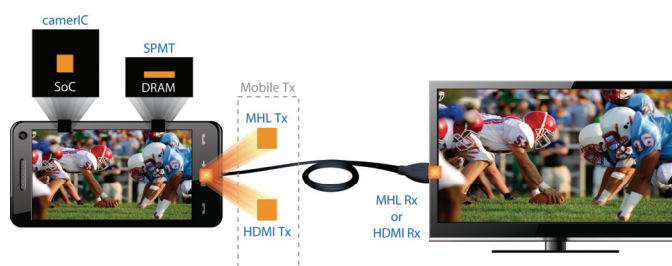
Figure 4: End-to-end HD solution for mobile applications
