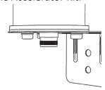
3. Tighten the screws until the antenna is firmly mounted against the building.
